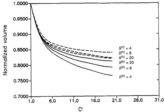
Fig. 3. Graph of the ensemble average “upper” and “lower” responses, normalized over the deterministic case  $C^i = C^m = 1$ .  $\delta^{(e)}$  and  $\delta^{(n)}$  correspond to  $C_\delta^e$  and  $C_\delta^n$  in eqn. (15), respectively.
